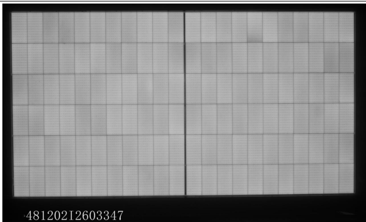
EL picture of Sample 03 after Ammonia test
