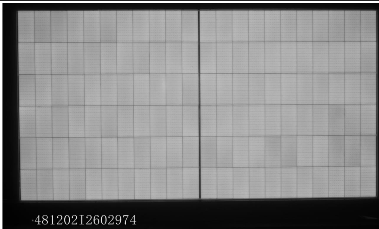
EL picture of Sample 02 after Ammonia test
